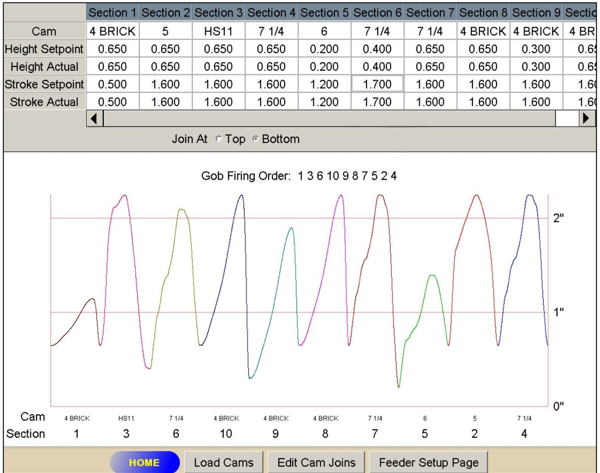
**Figure 14:** Once check box for Multi-Cam mode is checked, this screen appears, allowing input of sub cams.
