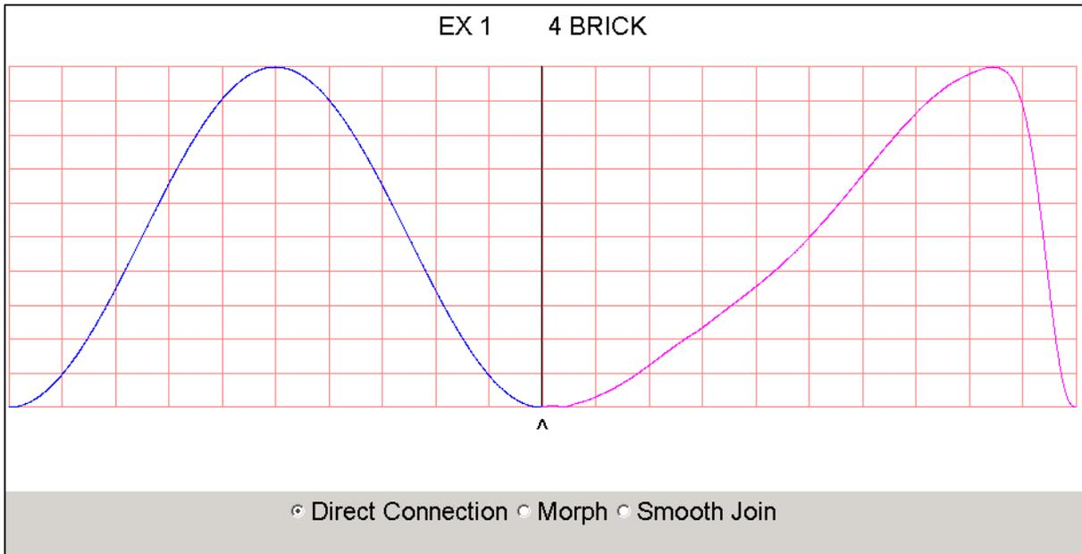
**Figure 9: Cams EX 1 and 4 BRICK connected at bottom with Direct Connection**
