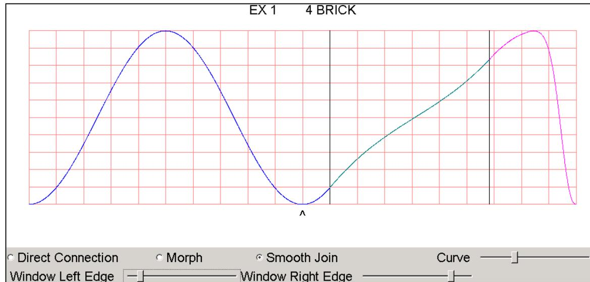
**Figure 12: Cams EX 1 and 4 BRICK connected at bottom with Smooth Join over a reduced window**
