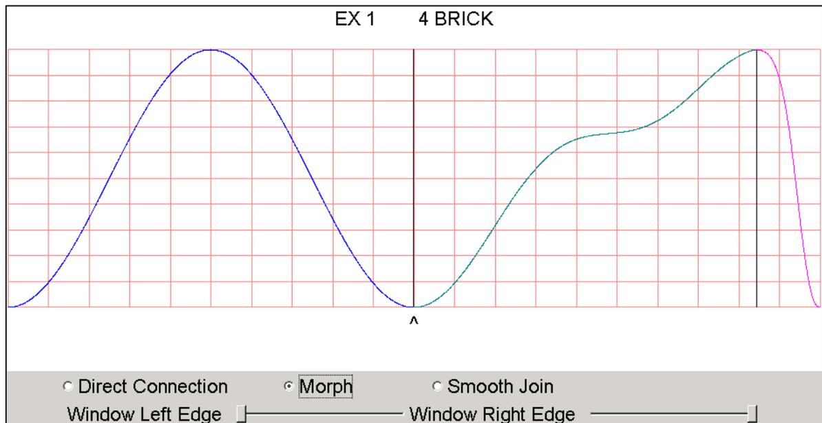
**Figure 10: Cams EX 1 and 4 BRICK connected at bottom with Morph over full window**
