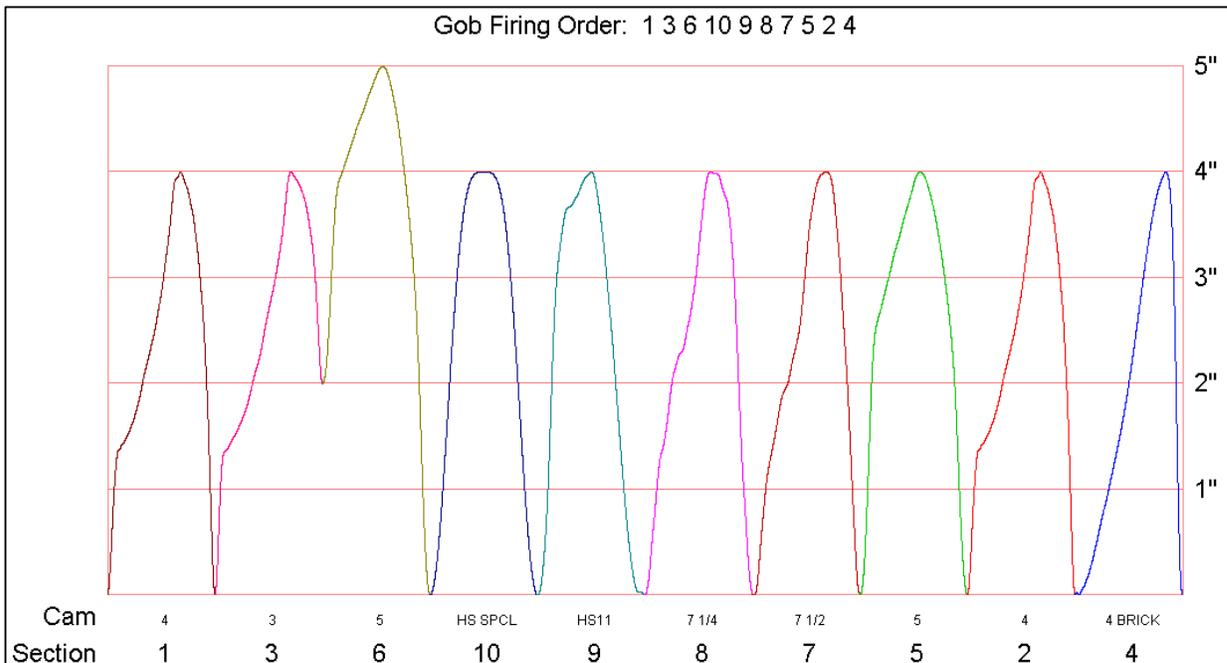
**Figure 7: Cam arrangement for a 10-section feeder with bottom-joined cams**
