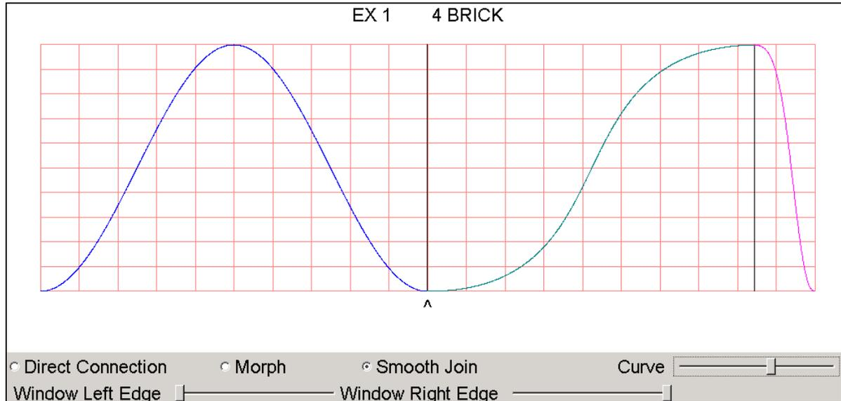
**Figure 11: Cams EX 1 and 4 BRICK connected at bottom with Smooth Join over full window**
