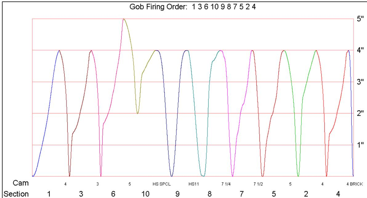
**Figure 8: Cam arrangement for a 10-section feeder with top-joined cams**
