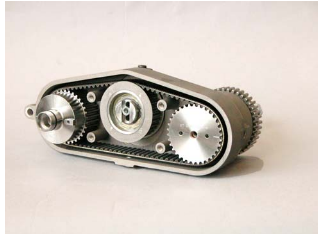
Figure 1 - Takeout Tong Arm, Wide Belt version (shown without cover)
