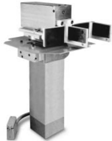
Pocket Air Finger assembly on an Emhart 860 Pusher System.
