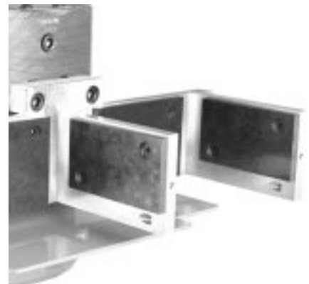
Closeup of Pocket Air Finger on a double gob installation. Note the inward facing air vents in the lower right corner of each finger.
