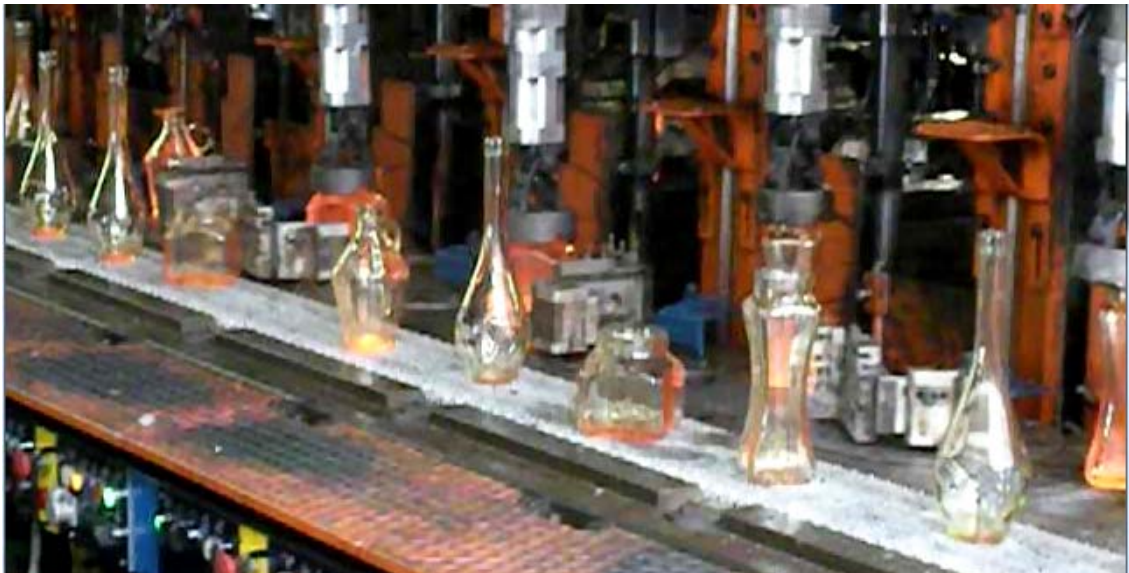
Versatility shown by 4 different containers (weight) on an 8 Section machine
