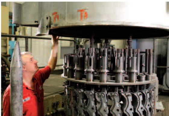
THE PLANT'S IONITRIDING CELLS USE GLOW DISCHARGE TECHNOLOGY TO ENSURE EXTRA-HARD METAL SURFACES
