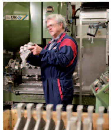
CHECKING A BATCH OF TRIPLE GOB TAKEOUT TONG HEADS
