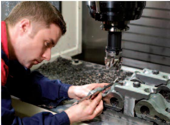
CHECKING THE SET-UP OF A MACHINING OPERATION
