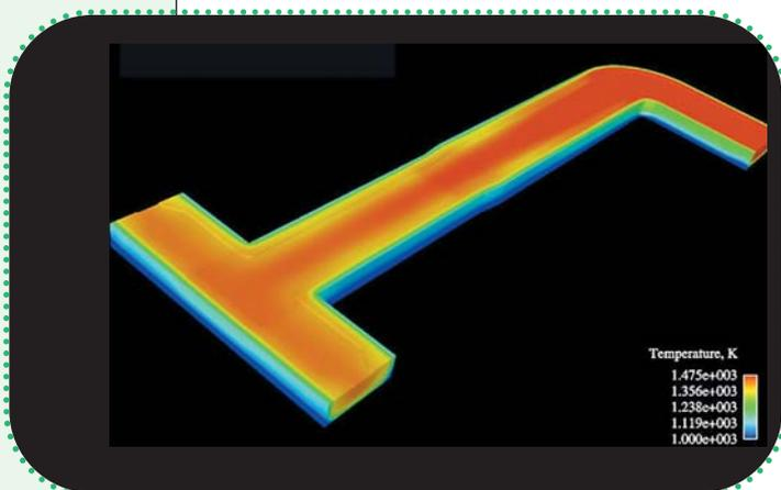
A numerical investigation has been carried out on the flow and thermal conditions of molten glass during its passage through the forehearth, a double gob feeder, delivery equipment, and finally through the container forming process of an IS machine. Of particular interest were the impacts of the forehearth exit plane temperature on the final container quality.
