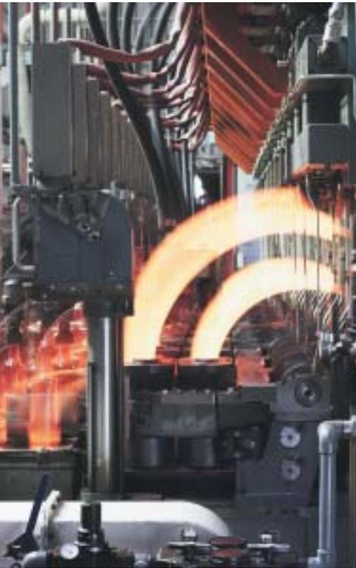
only fully servo-electric-driven IS machine on the market. Both the AIS and NIS machines have the advantage of parallel mold motion, and they also open up the possibility of achieving more effective production of standard glass containers through the triple-gob production method. The NIS can also operate in quadruple-gob mode.
