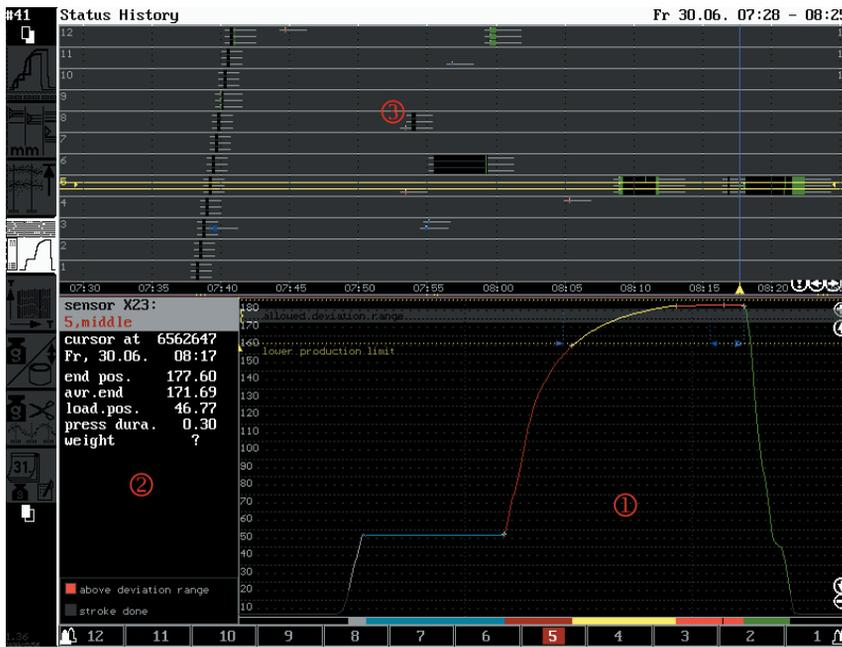
The Status History screen virtualizes the selected plunger stroke. gray: reverse position – white: motion into loading position – blue: stop in loading position – dark red: fast upward to press – yellow: transition into final press – light red: final press – green: fast downward to reserve position
