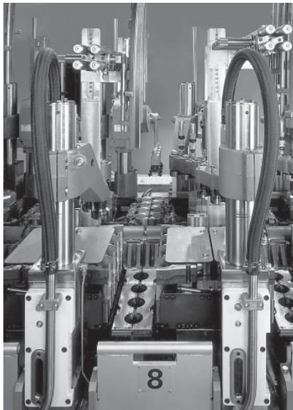
**The NIS machine features parallel mold open and close mechanisms on both the blank side and blow side (shown here in quad gob configuration), which enables more precise control of blank and blow mold movements.** Photo: Emhart Glass
