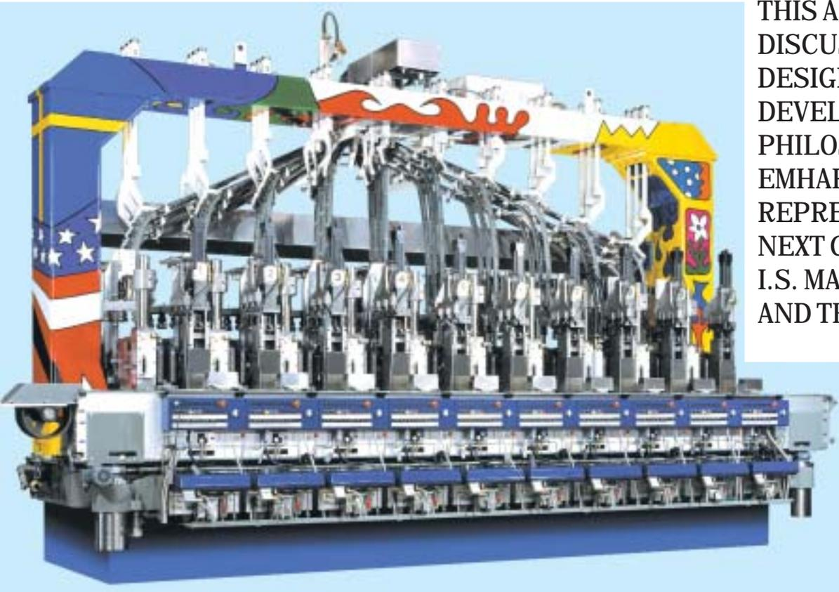
**T**he NIS Machine and Controls system was introduced in 2000 with the goal of setting the next standard for glass forming machines and for future investment in the glass container forming industry. In addition to the high capacity for which the 5-inch triple gob machine was designed, the NIS provides a platform for the state-of-the-art process control that Emhart Glass believes is needed in the glass industry.
