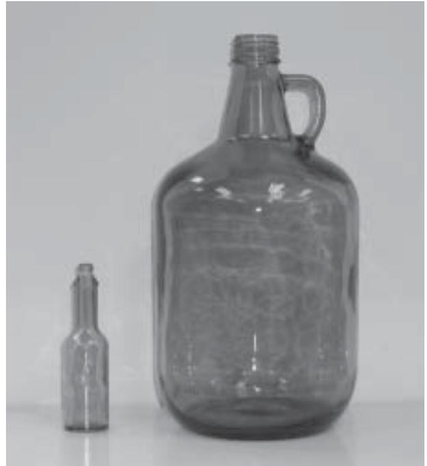
**Figure 3.** Range of containers produced on a Single 340 Forehearth
