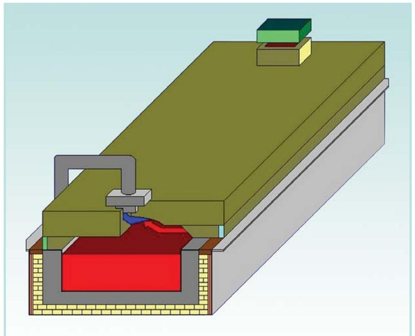
trol the amount of heat taken from or input to the glass. Cooling the forehearth superstructure will therefore produce glass cooling; selectively cooling different parts of the forehearth superstructure by different degrees, however, will produce glass conditioning.
