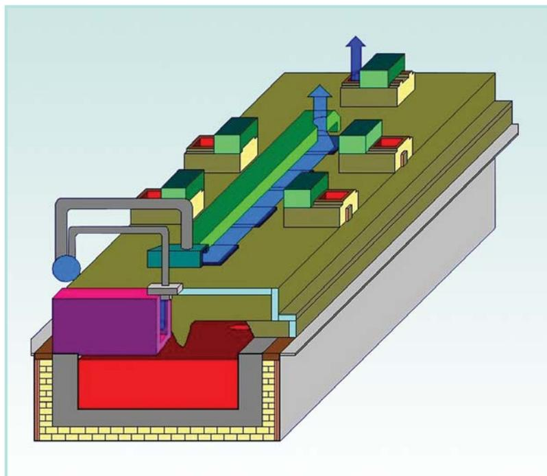
tem transitions into heating mode, the cooling air flow rate to the dual cooling system will lessen and the central and side damper openings will decrease. The system is configured so that although all side dampers are closed when operated in heating mode, the central damper remains partially open to facilitate the exhaust of the combustion gases.
