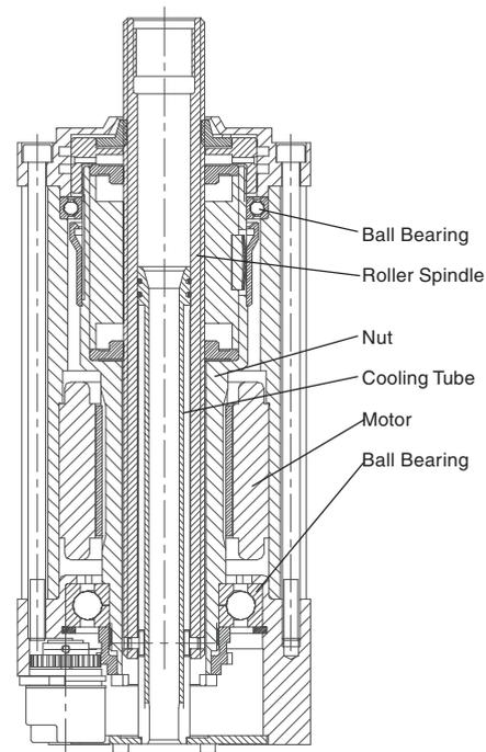
Figure 1. Drawing of mechanism
