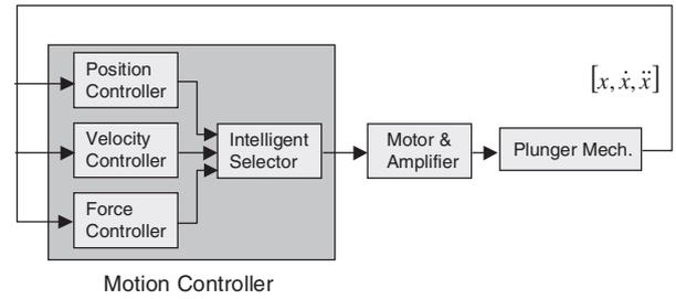
Figure 6. Block diagram of model with motion controller
