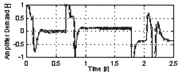
Figure 10. Measured (dashed line with crosses) and simulated (solid line) controller output for trial with glass
