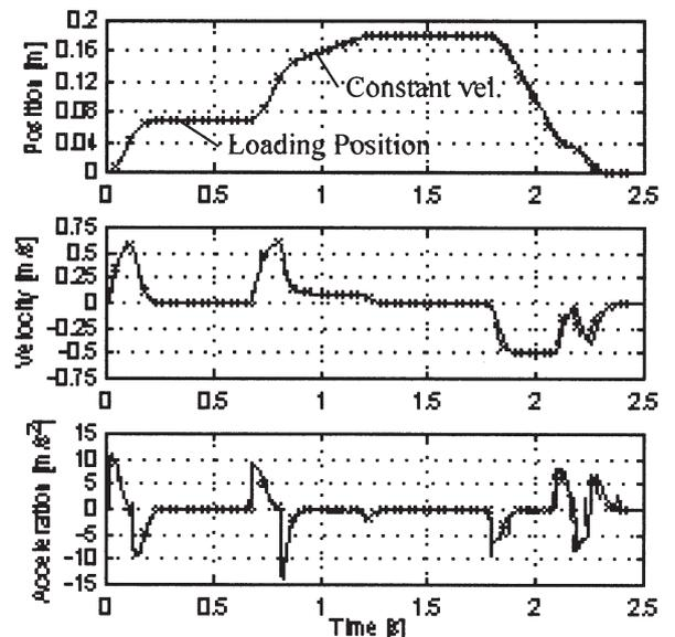
Figure 7. Measured (dashed line with crosses) and simulated (solid line) position, velocity and acceleration of plunger without glass
