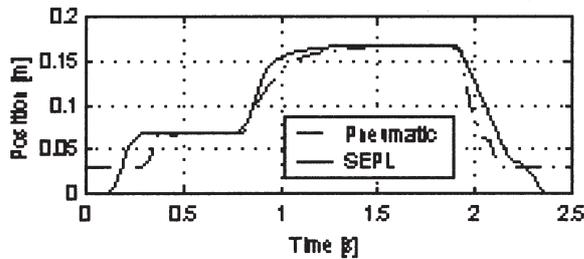
**Figure 11.** Comparison between pneumatic and servo-electric plunger mechanism
