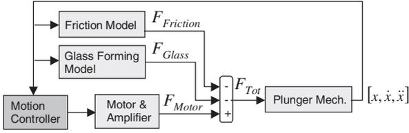
Figure 2. Simplified block diagram of model
