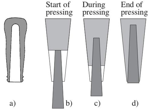
Figure 4. Shape of typical parison a) and model of parison at different press phases b)–d)
