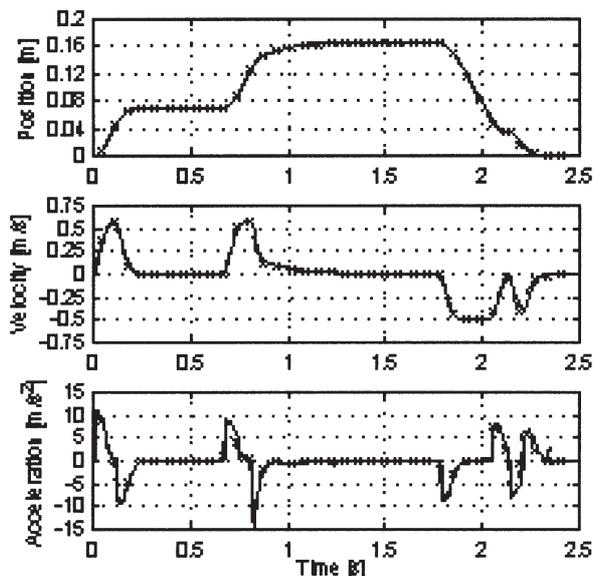
Figure 9. Measured (dashed line with crosses) and simulated (solid line) position, velocity and acceleration of plunger with glass
