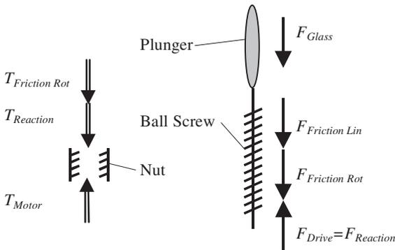
Figure 3. Driving and friction forces
