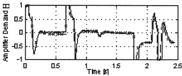
Figure 8. Measured (dashed line with crosses) and simulated (solid line) controller output for trial without glass
